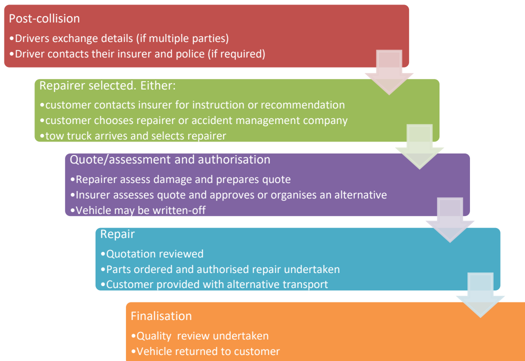
Figure 2: Repair process overview
